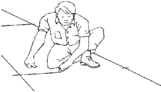
**FIGURE 6: Mark Floor Level Difference**
