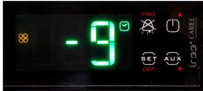
The Carel IR33+ controller has a two-level menu system for programming the operation of the case; Level 1 and Level 2 program settings. Unlike IR33, the IR33+ control system is easier to use with a password.
