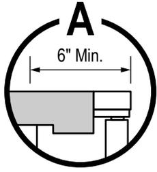
Building soffits must be set back at least 6" from the front of the doors to allow access to electrical wiring on the top of the case.
