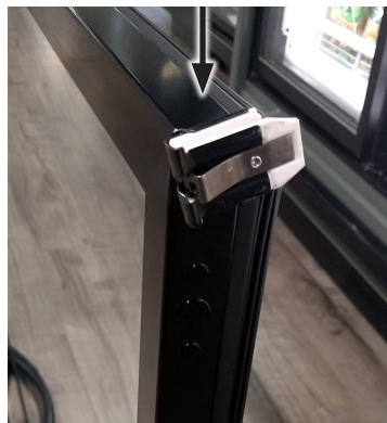
FIGURE 28: Remove Hinge Pin
